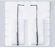
Five pieces are stacked each on left and right of the backing paper, wrapped and fixed.
